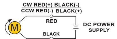
The direction of motor rotation is as viewed from the front shaft end of the motor. Matching Gear Ratio 1:3 to 1:250 & Decimal Gear available.
